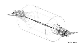
Figure 3. Fundamental bending mode shape of model scale compulsator rotor at zero speed.
