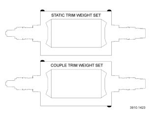
Figure 8. Location of balance weights for static (top) and couple (bottom) trim balance corrections.
