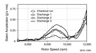
Figure 10. Vibration data for the model scale compulsator rotor for all runs conducted to date to its maximum design speed of 12,000 rpm.
