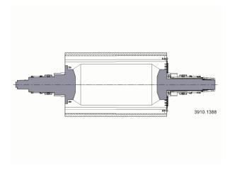
Figure 1. Model scale compulsator rotor.
